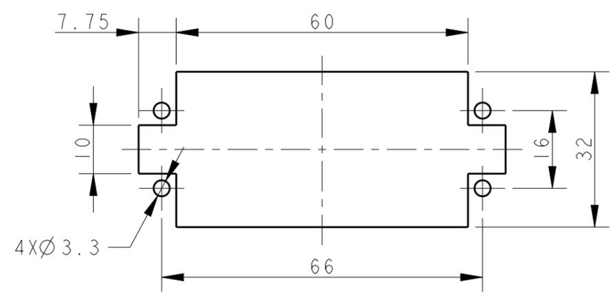
PANEL CUT OUT DIMENSION FOR INSERT WITHOUT HOODS/HOUSING, ONLY FOR REFERENCE
