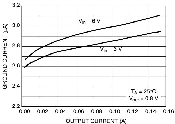
**Figure 3. Ground Pin Current vs. Output Current**
