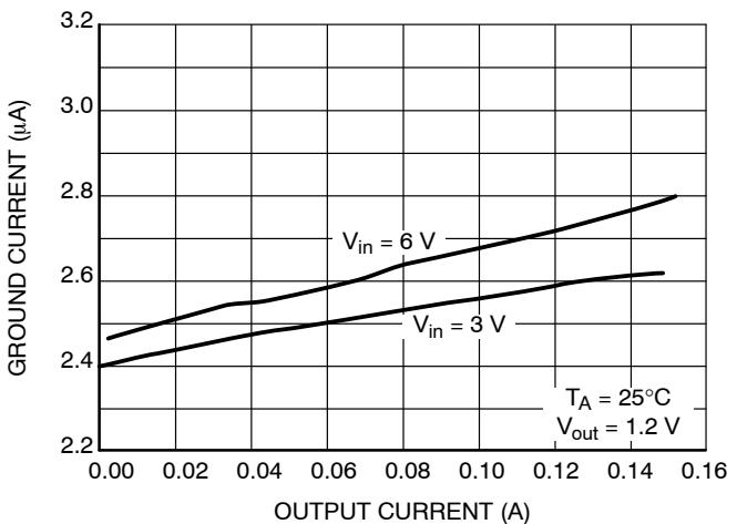
**Figure 4. Ground Pin Current vs. Output Current**
