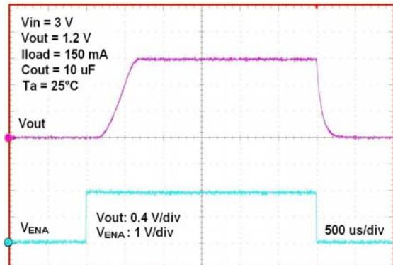
Figure 18. Enable Operation
