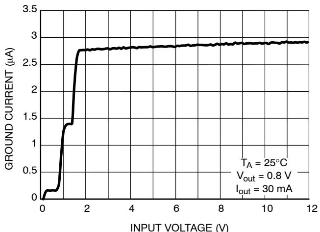
**Figure 7. Ground Pin Current vs. Input Voltage**
