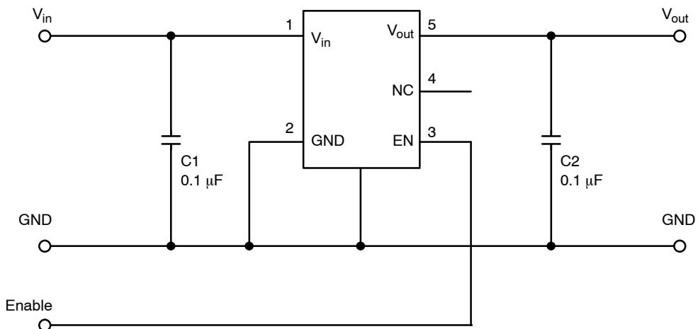
Figure 2. Typical Application Schematic for TSOP-5 Package
