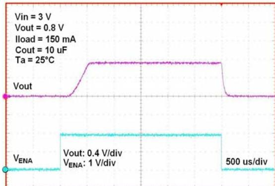
Figure 17. Enable Operation
