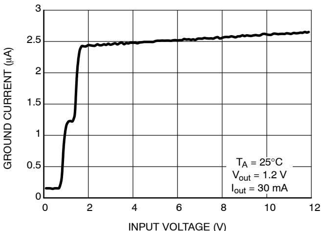
**Figure 8. Ground Pin Current vs. Input Voltage**
