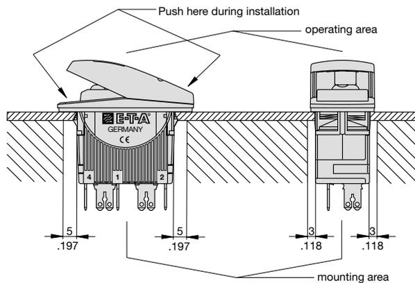
This is a metric design and millimeter dimensions take precedence ( $\frac{\text{mm}}{\text{inch}}$ )
