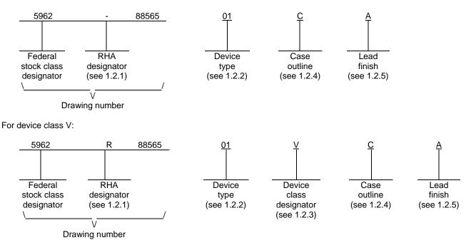
1.2.1 <u>RHA designator</u>. Device classes Q and V RHA marked devices meet the MIL-PRF-38535 specified RHA levels and are marked with the appropriate RHA designator. Device class M RHA marked devices meet the MIL-PRF-38535, appendix A specified RHA levels and are marked with the appropriate RHA designator. A dash (-) indicates a non-RHA device.
