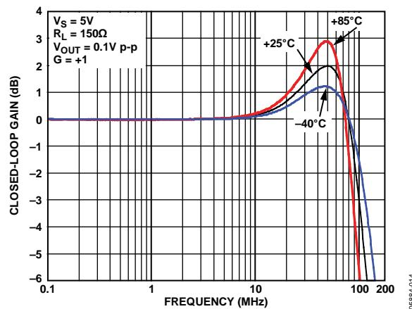
Figure 16. Small Signal Frequency Response for Various Temperatures
