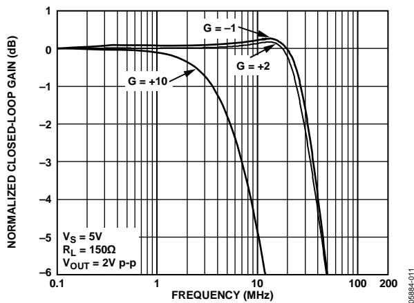
Figure 13. Large Signal Frequency Response for Various Gains
