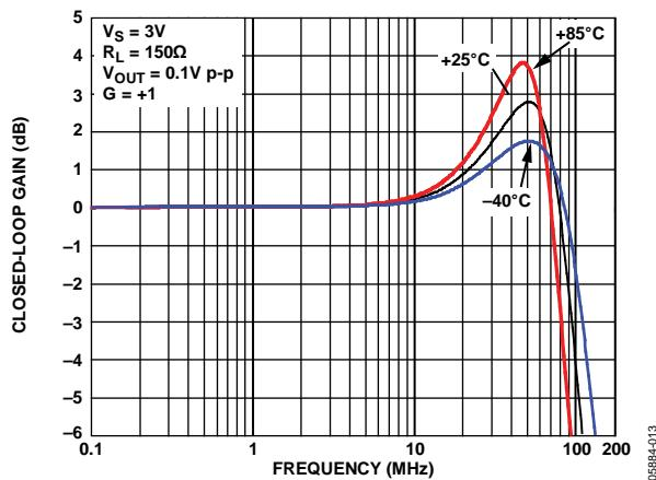
Figure 15. Small Signal Frequency Response for Various Temperatures
