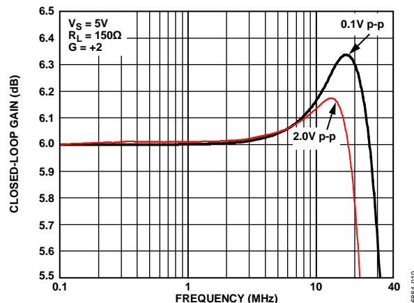
Figure 11. 0.5 dB Flatness Response for Various Output Voltages
