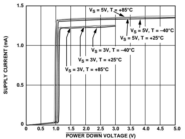
Figure 38. Supply Current vs. POWER DOWN Voltage
