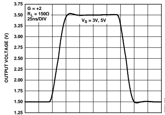
Figure 30. Large Signal Pulse Response for Various Supplies
