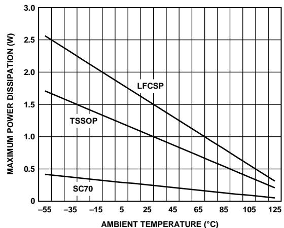
Figure 6. Maximum Power Dissipation vs. Temperature for a 4-Layer Board
