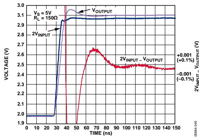
Figure 46. 0.1% Settling Time
