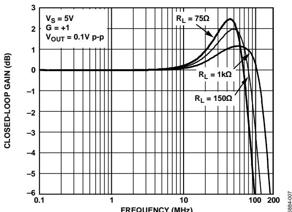
Figure 8. Small Signal Frequency Response for Various Loads
