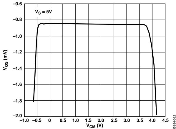
Figure 50.  $V_{OS}$  vs. Common-Mode Voltage,  $V_S = 5\text{ V}$
