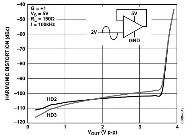
Figure 27. Harmonic Distortion for Various Output Voltages
