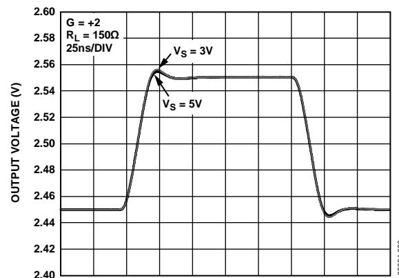
Figure 28. Small Signal Pulse Response for Various Supplies
