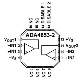
Figure 2. 16-Lead LFCSP\_VQ
