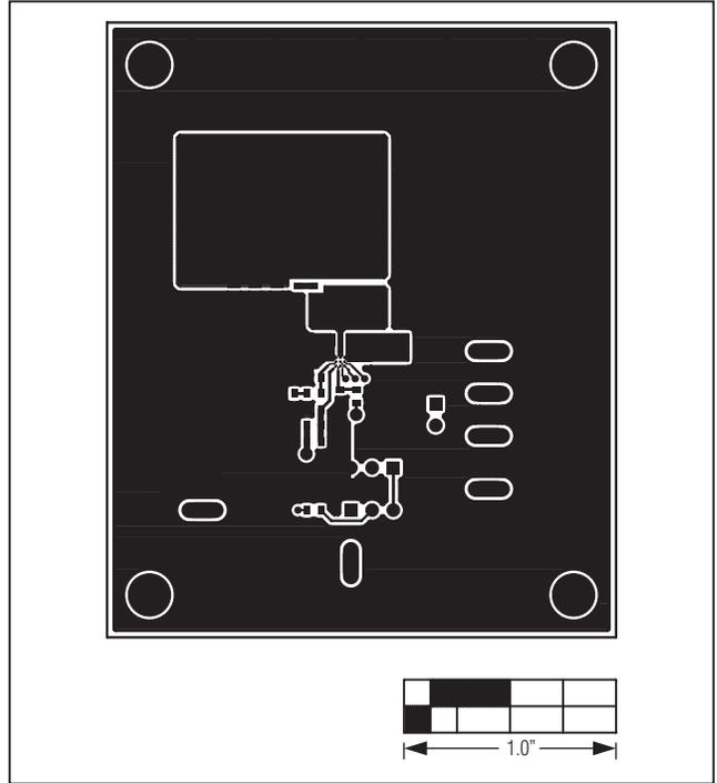
Figure 3. MAX15058 EV Kit Component PCB Layout—Component Side
