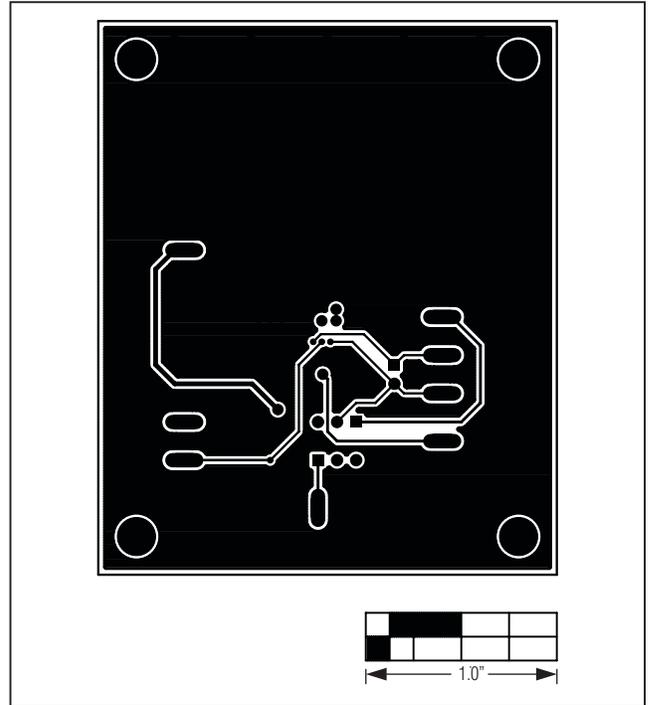
Figure 6. MAX15058 EV Kit PCB Layout—Solder Side
