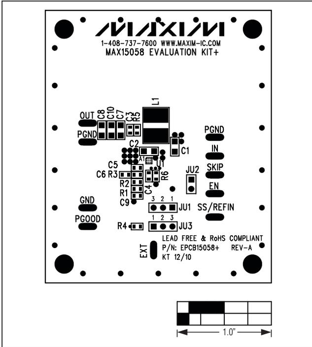
Figure 2. MAX15058 EV Kit Component Placement Guide—Component Side
