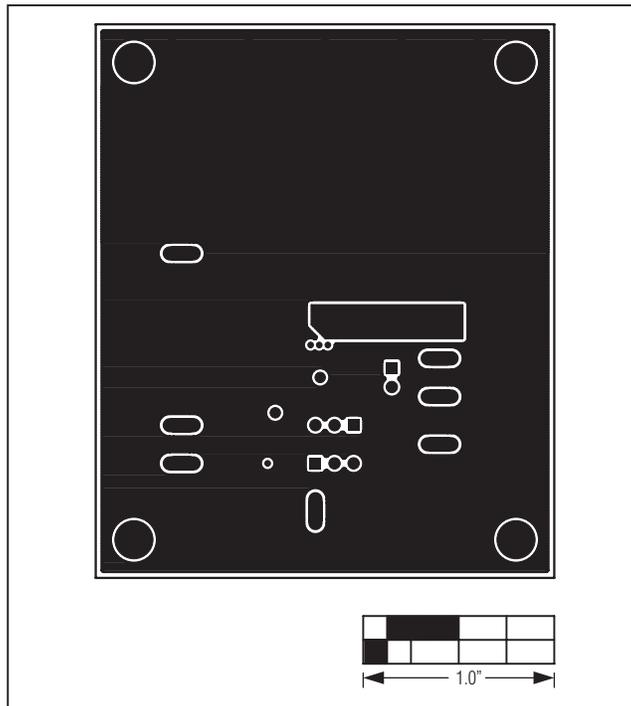
Figure 4. MAX15058 EV Kit PCB Layout—Inner Layer 2
