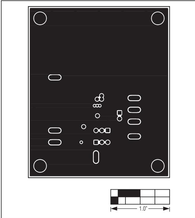
Figure 5. MAX15058 EV Kit PCB Layout—Inner Layer 3
