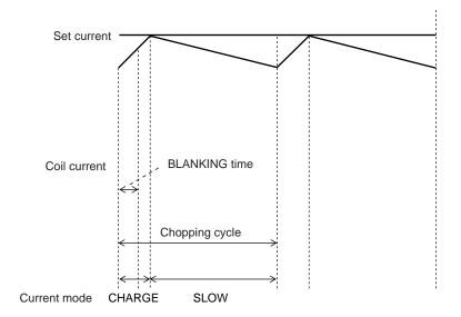
Based on the voltage input to the VREF pin and the resistance connected between RF and GND, the output current that is subject to the constant-current control is set using the calculation formula below:
