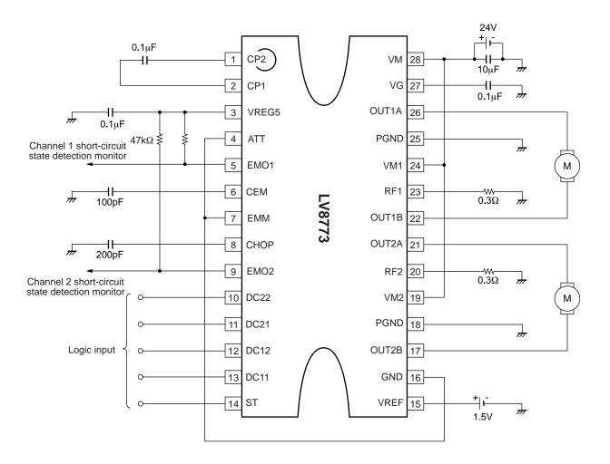
The formulae for setting the constants in the examples of the application circuits above are as follows: Constant current limit (100%) setting
