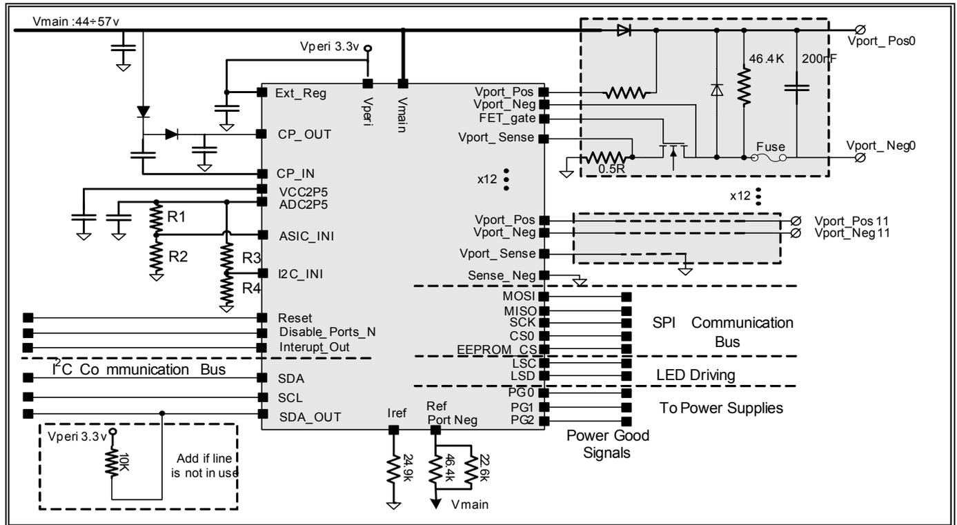
**Figure 4: Basic Application with AC Disconnect Support**
