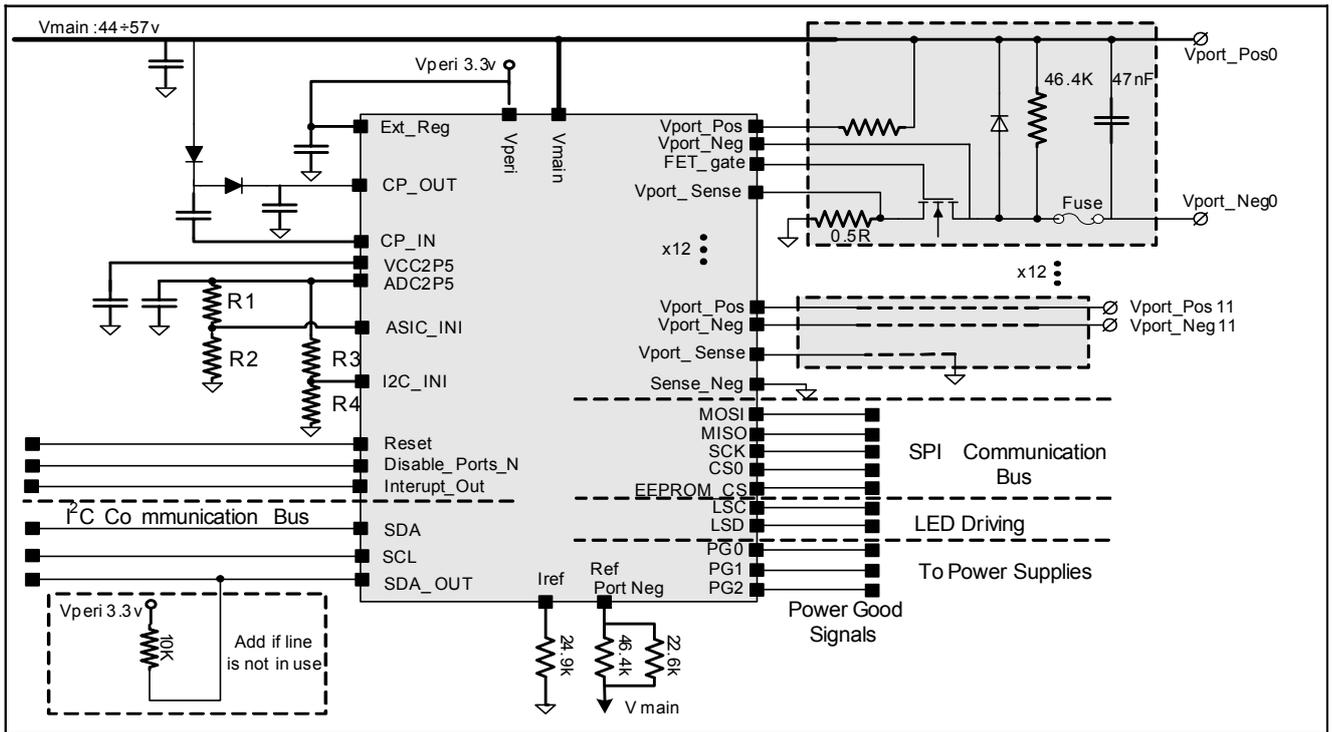
**Figure 5: Basic Application with DC Disconnect Support**
