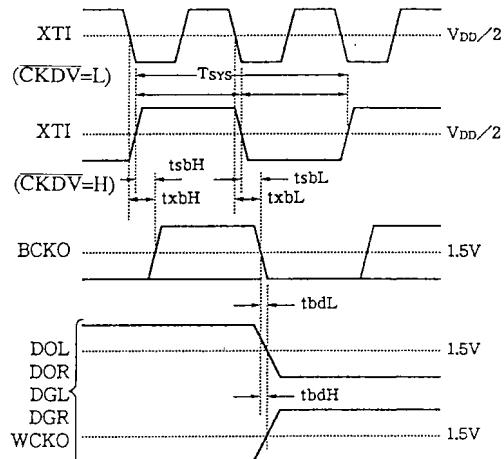
**SM5813APT/AF**(Ta = -20 to 70°C, V<sub>DD</sub> = 4.75 to 5.25V, V<sub>SS</sub> = 0V)**1. XTI TERMINAL****a. In case of crystal oscillation**
