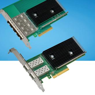
Dual and Quad –port 10GbE adapters supporting highly scalable iWARP RDMA for high-throughput, low-latency, and low-CPU data communication.
