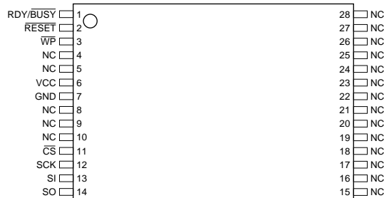
TSOP Top View – Type 1
