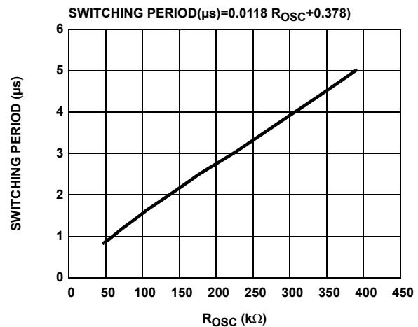
FIGURE 14.  $F_S$  vs  $R_{\text{OSC}}$ 100K & 0.1μF DELAY NETWORK ON ENP,  $C_{\text{SS}}=0.1\mu\text{F}$
