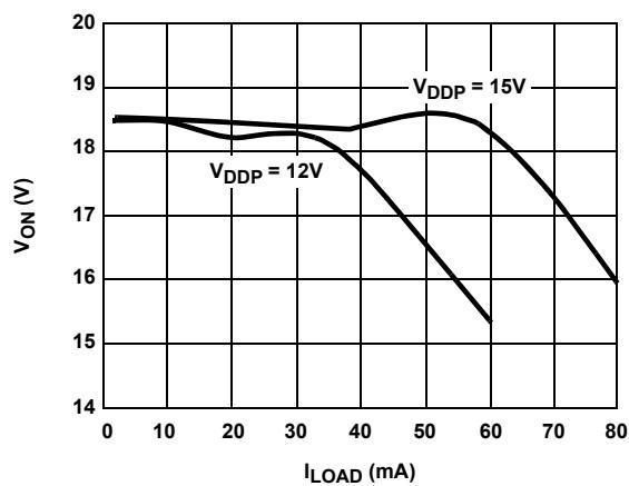
FIGURE 11. V<sub>ON</sub> vs I<sub>ON</sub>
