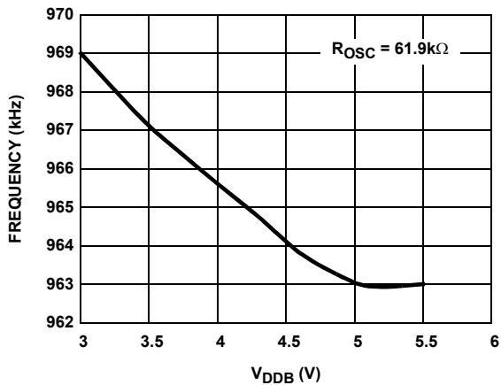
FIGURE 5.  $F_S$  vs  $V_{DDB}$
