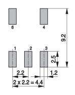
Recommended PCB layout (top view)
