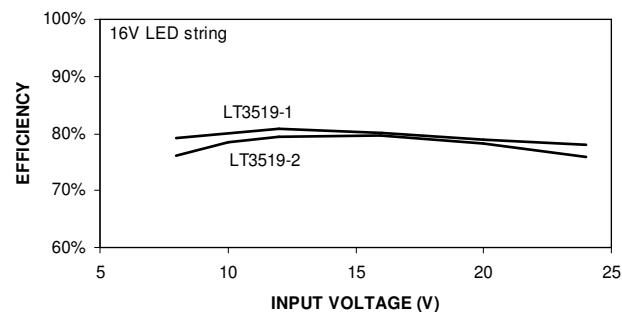
Figure 1. DC1612A Efficiency vs. PVIN 16VLED 150mA
