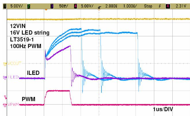
Figure 2. DC1612A-A 16VLED PWM Dimming PVIN=12V
