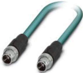
Assembled Ethernet cable, CAT6 A shielded, 4-pair, AWG 26 stranded (7-wire), RAL 5021 (water blue), M12 connector on M12 connector, length 20 m
