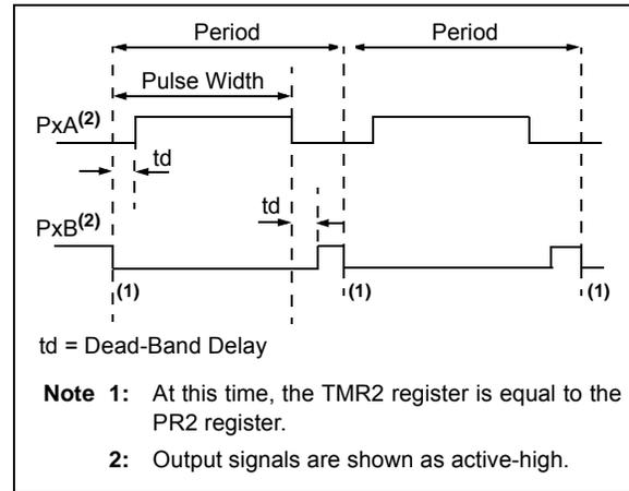
**FIGURE 20-7: EXAMPLE OF HALF-BRIDGE APPLICATIONS**
