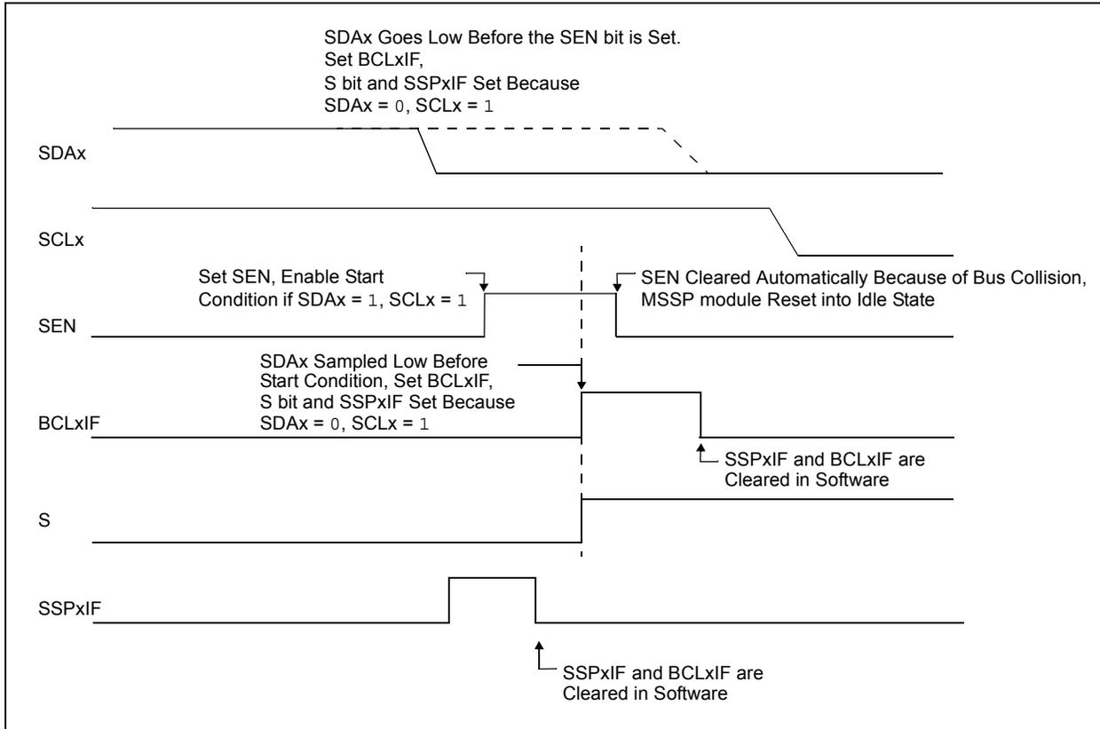
**FIGURE 21-29: BUS COLLISION DURING START CONDITION (SCLx = 0)**
