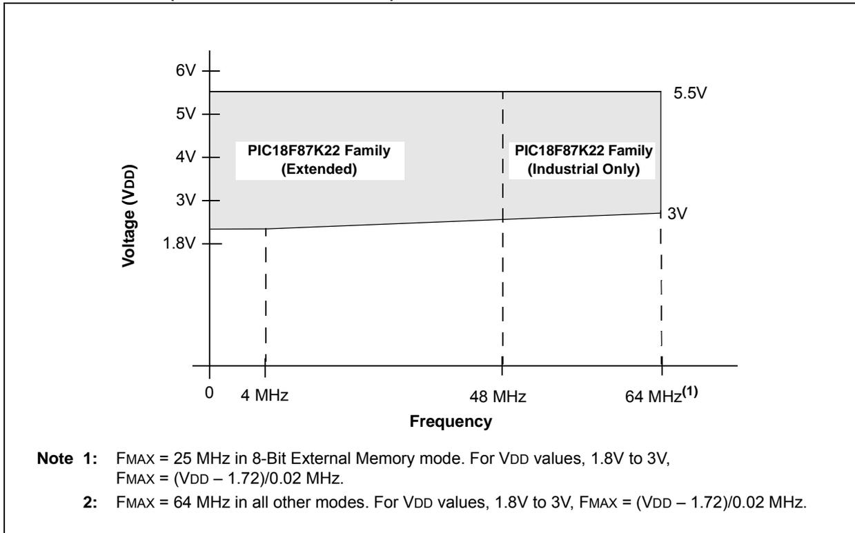
**FIGURE 31-2: VOLTAGE-FREQUENCY GRAPH, REGULATOR DISABLED (INDUSTRIAL/EXTENDED)<sup>(1,2)</sup>**
