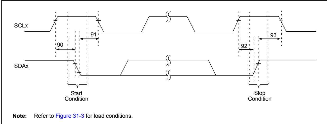
**TABLE 31-21: I<sup>2</sup>C™ BUS START/STOP BITS REQUIREMENTS (SLAVE MODE)**
