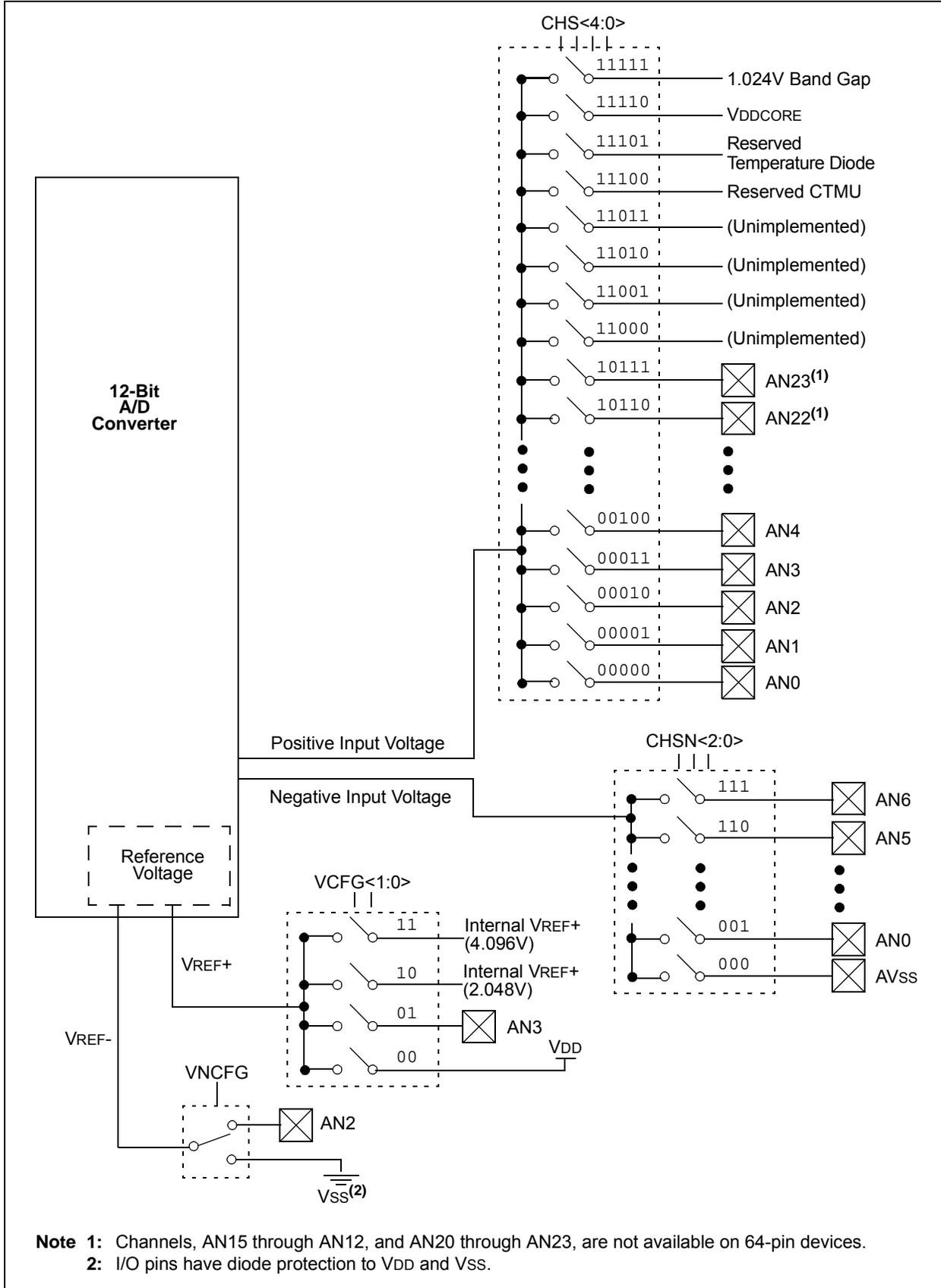
**Note 1:** Channels, AN15 through AN12, and AN20 through AN23, are not available on 64-pin devices.
