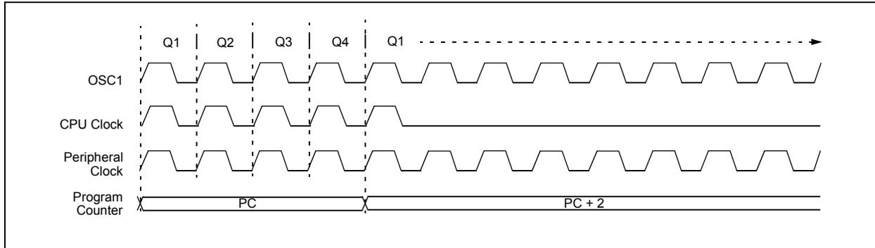
**FIGURE 4-8: TRANSITION TIMING FOR WAKE FROM IDLE TO RUN MODE**
