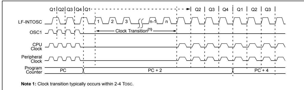
**FIGURE 4-4: TRANSITION TIMING FROM RC\_RUN MODE TO PRI\_RUN MODE**
