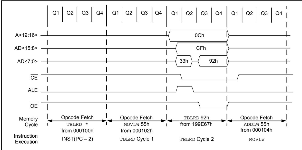
**FIGURE 8-8: EXTERNAL MEMORY BUS TIMING FOR SLEEP (EXTENDED MICROCONTROLLER MODE)**
