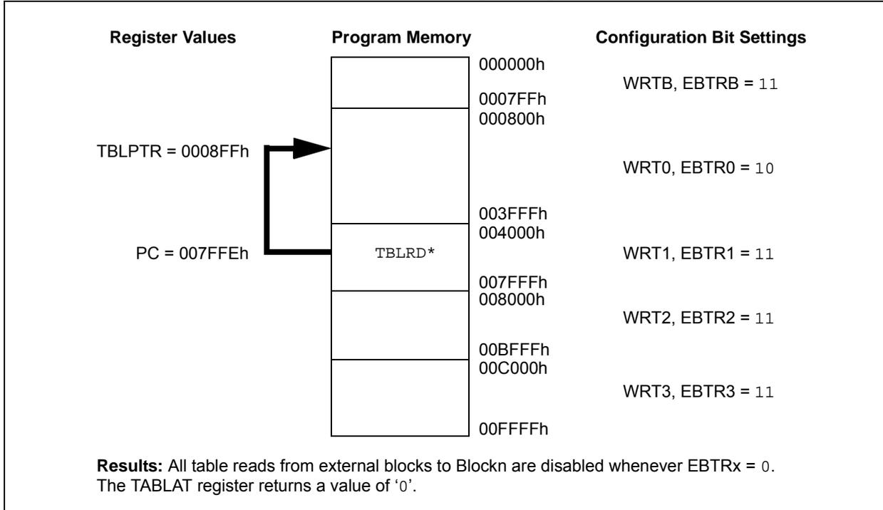
**FIGURE 28-9: EXTERNAL BLOCK TABLE READ (EBTRx) ALLOWED**
