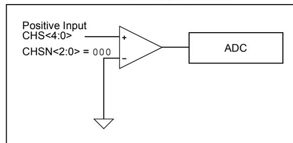
In the Single Channel Measurement mode, the negative input is connected to AVSS by clearing the CHSN bits (ADCON1<2:0>).
