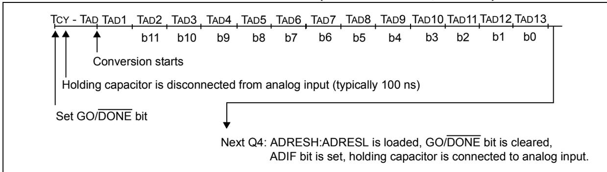
**FIGURE 23-7: A/D CONVERSION TAD CYCLES ( $\text{ACQT}<2:0> = 010, \text{TACQ} = 4 \text{TAD}$ )**
