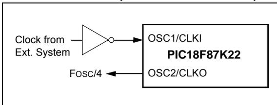
An external clock source may also be connected to the OSC1 pin in HS mode, as shown in [Figure 3-6](#). In this configuration, the divide-by-4 output on OSC2 is not available. Current consumption in this configuration will be somewhat higher than EC mode, as the internal oscillator's feedback circuitry will be enabled (in EC mode, the feedback circuit is disabled).
