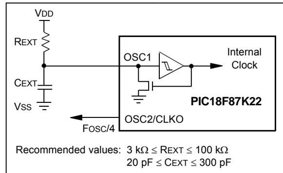
The RCIO Oscillator mode (**Figure 3-3**) functions like the RC mode, except that the OSC2 pin becomes an additional general purpose I/O pin. The I/O pin becomes bit 6 of PORTA (RA6).
