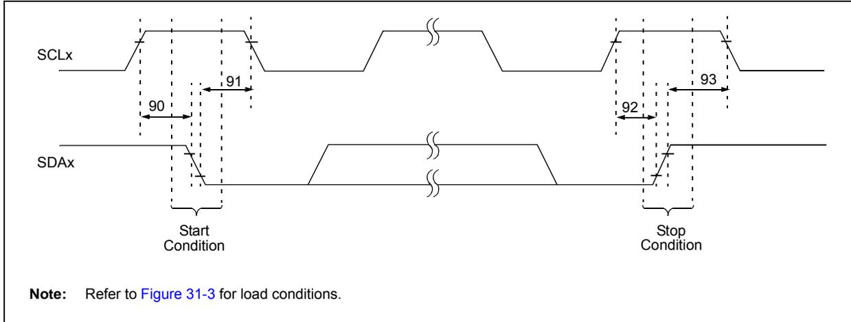
**TABLE 31-23: MSSP I<sup>2</sup>C™ BUS START/STOP BITS REQUIREMENTS**
