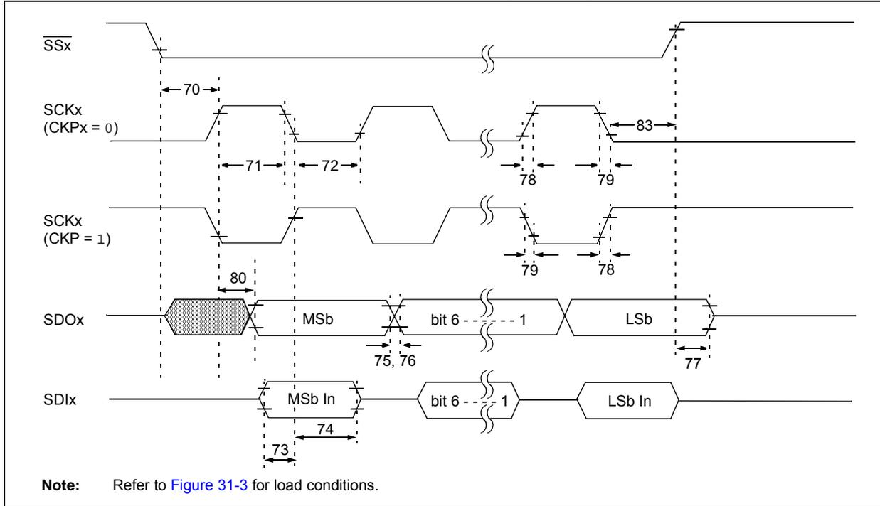
**TABLE 31-19: EXAMPLE SPI MODE REQUIREMENTS (SLAVE MODE TIMING, CKE = 0)**
