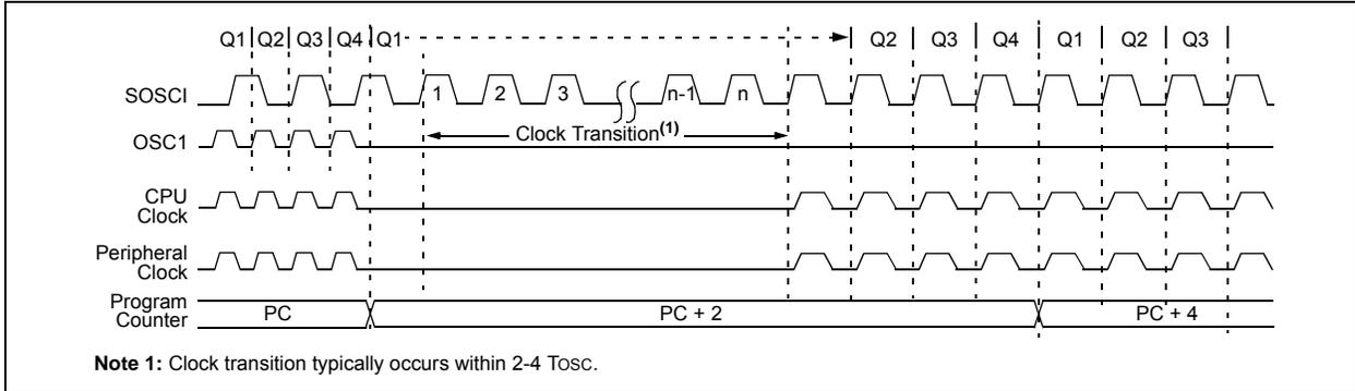
**FIGURE 4-2: TRANSITION TIMING FROM SEC\_RUN MODE TO PRI\_RUN MODE (HSPLL)**
