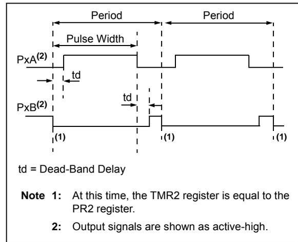
**FIGURE 20-15: EXAMPLE OF HALF-BRIDGE APPLICATIONS**
