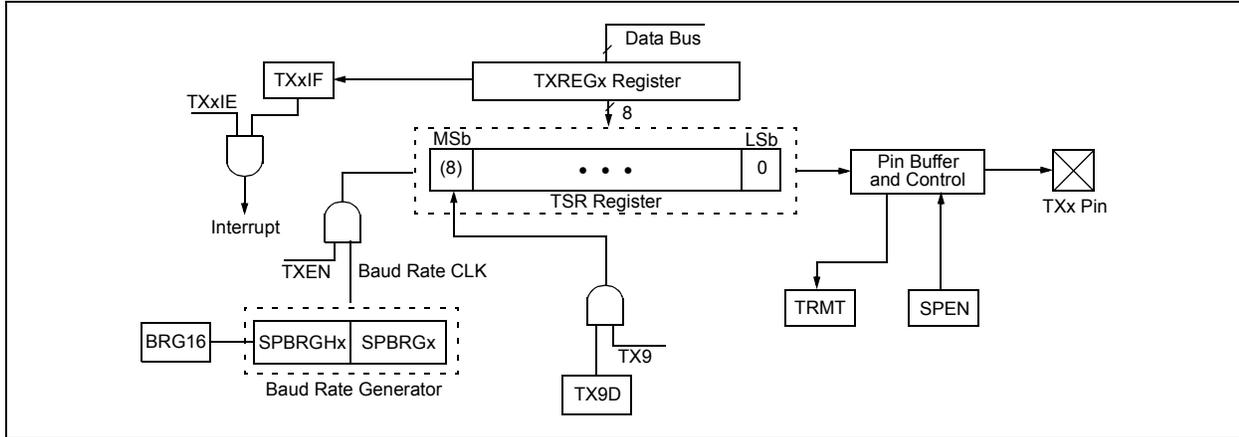
**FIGURE 22-4: ASYNCHRONOUS TRANSMISSION**
