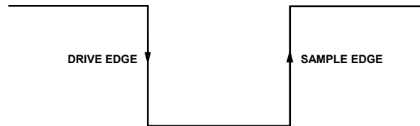
Figure 78. SPI Mode 0 SCLK Edges
