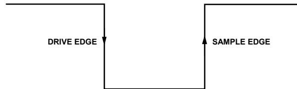
Figure 78. SPI Mode 0 SCLK Edges
