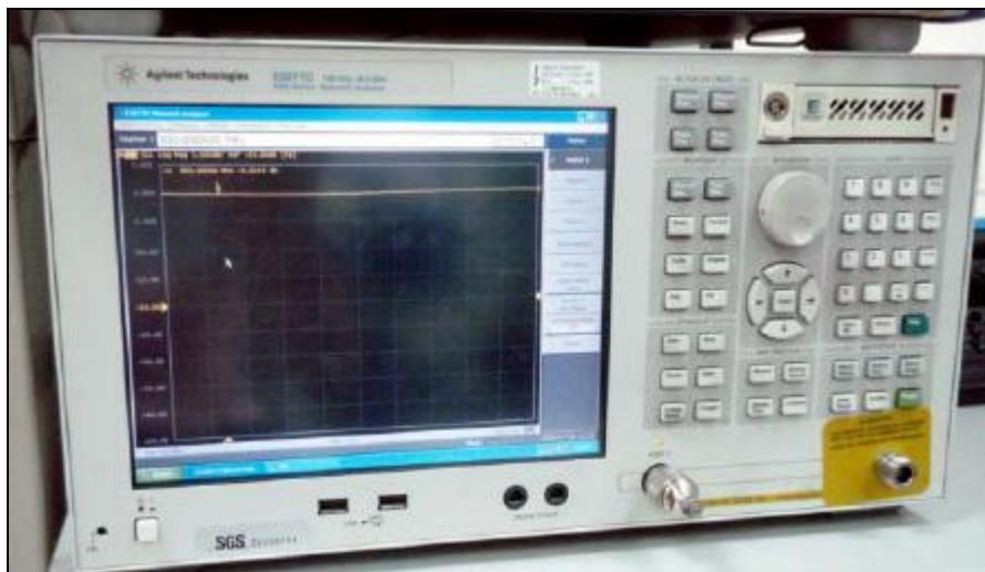
**Figure 2.** Network Analyzer.
