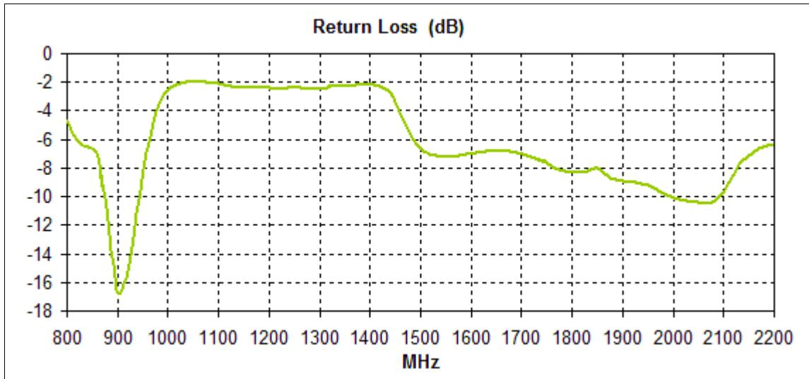
**Figure 3.** Return Loss for the FXP14 Antenna.
