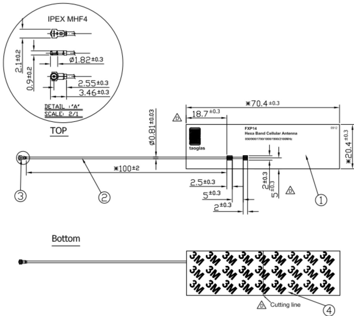
**Figure 9.** Mechanical Drawing for the FXP14 Antenna.
