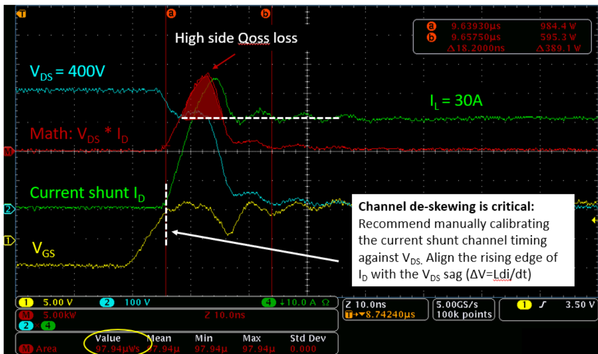
Figure 21 Turn-on switching loss measurement ( E_{on}=98\mu J , 400V/30A, T_J=25^\circ C )
