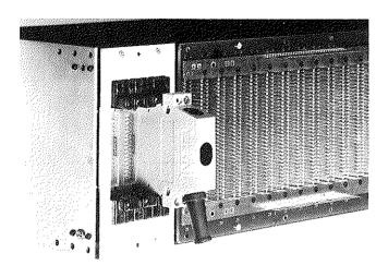
In a similar way to front-mounted connectors, this interface system also provides for making mateable interconnections directly from the wiring end to a printed circuit board. The guide elements are mounted on the mother board and serve to locate the card in the rack.
