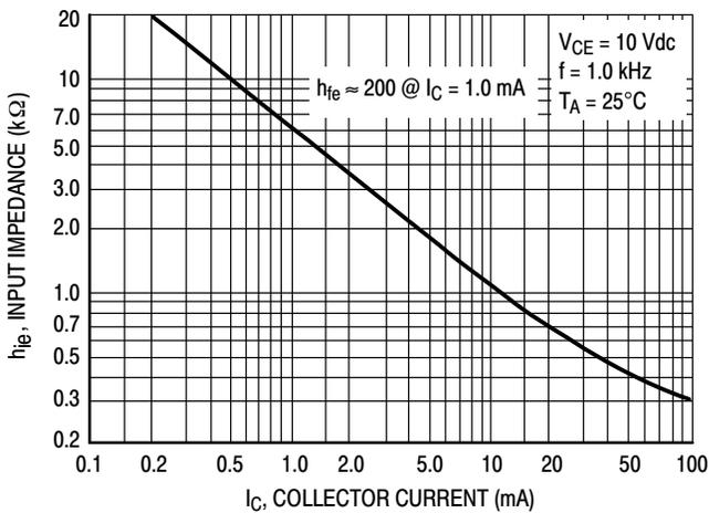
Figure 18. Input Impedance
