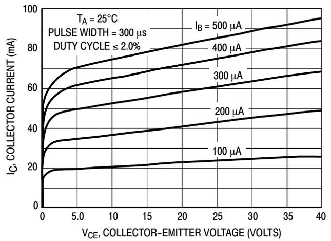
Figure 11. Collector Characteristics
