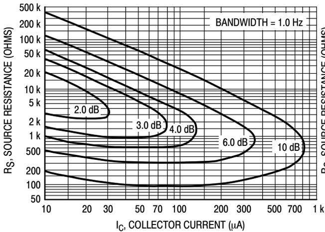
Figure 6. Narrow Band, 100 Hz
