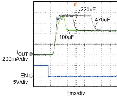
**1Ω Load Connected to Enabled Device**
