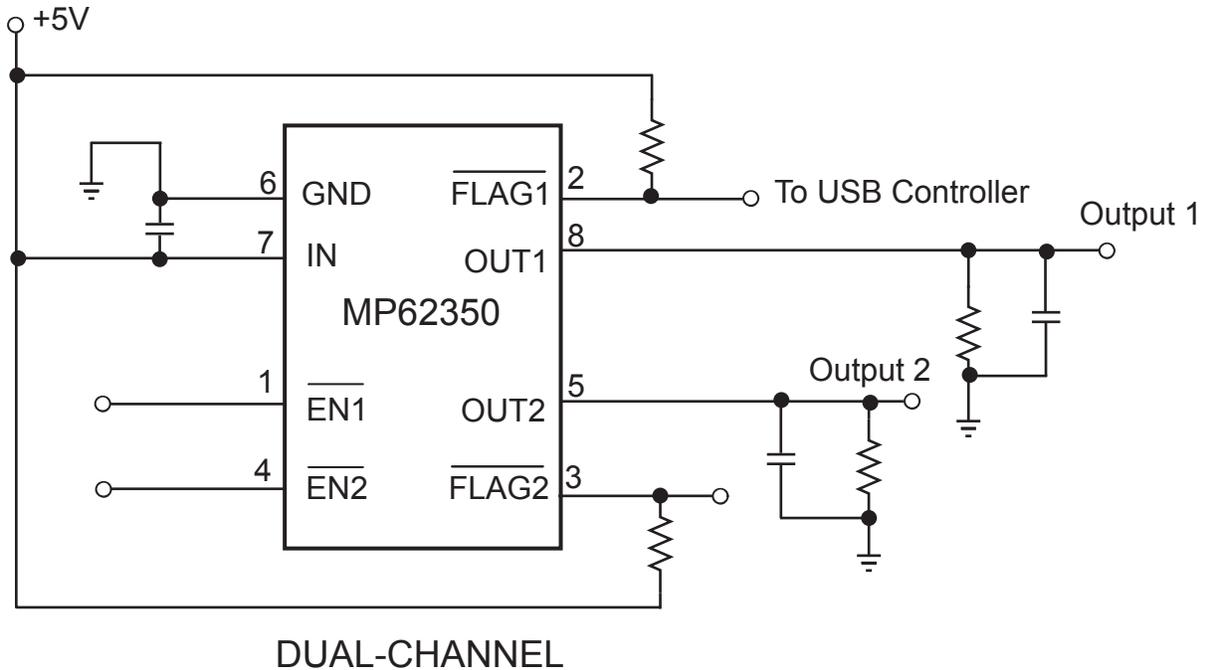
Figure 3—Application Circuit
