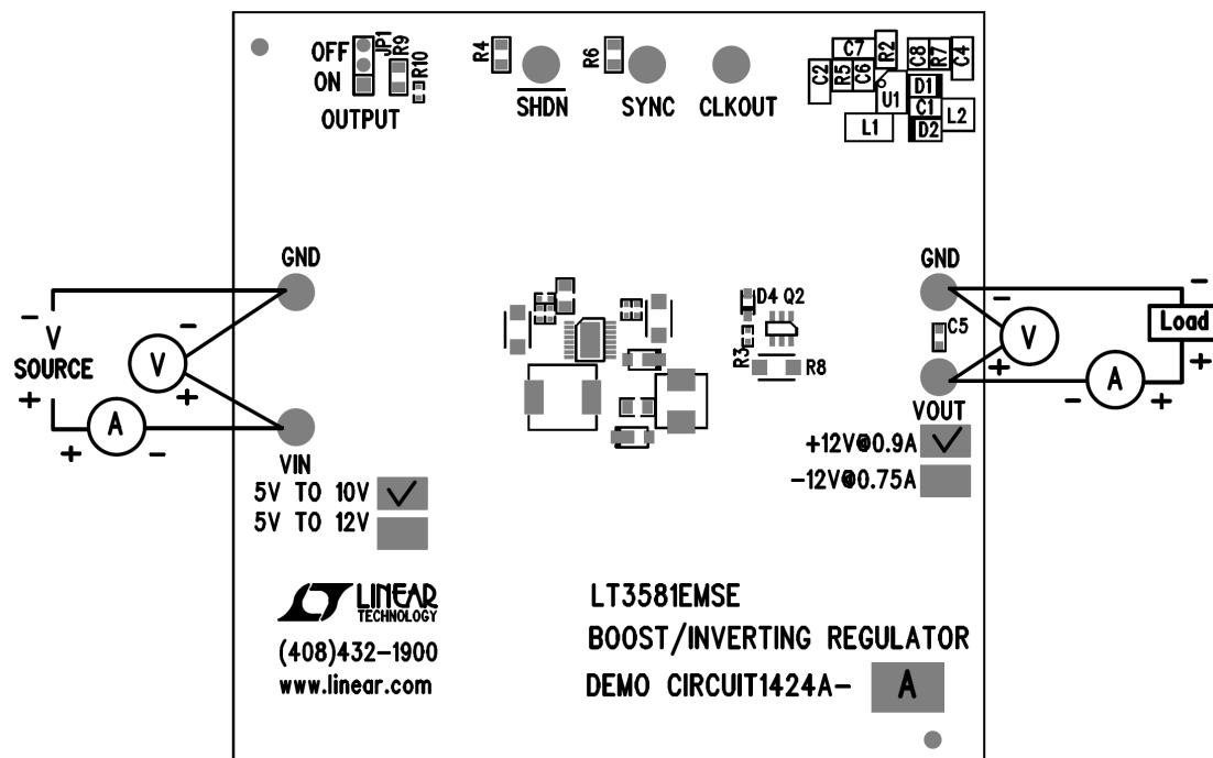
Figure 1. DC1424A-A Proper Equipment Setup
