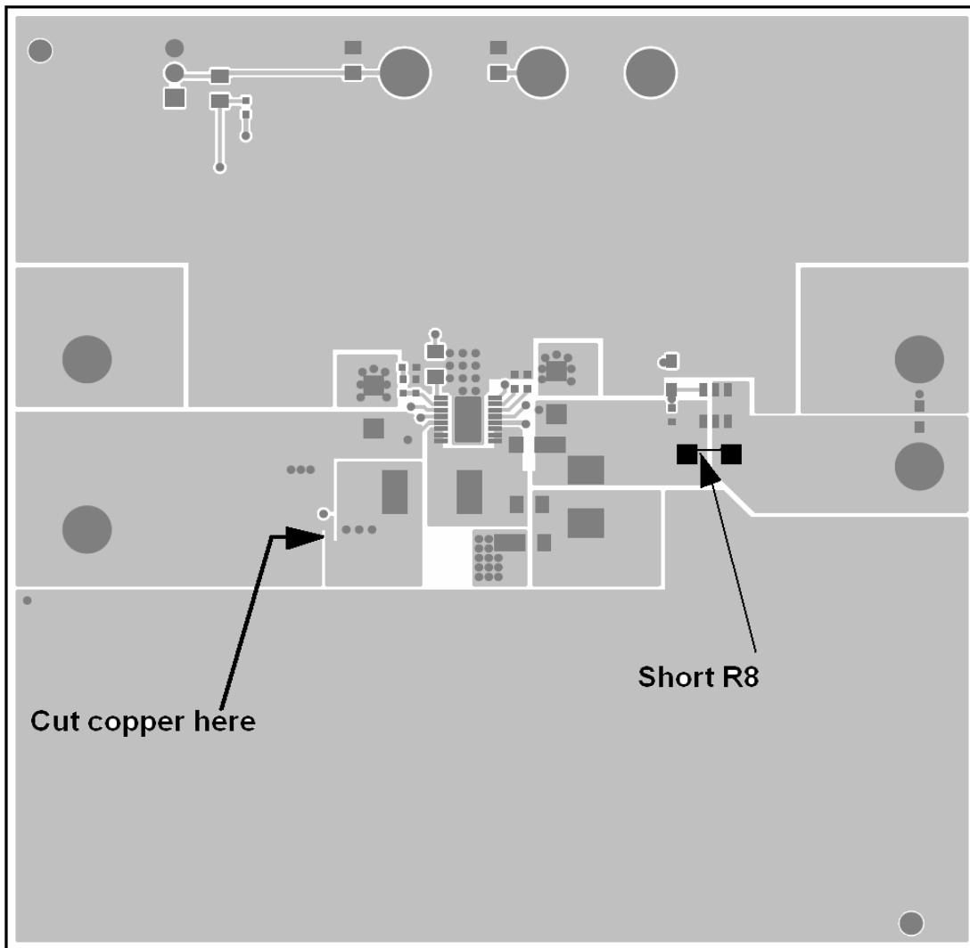
Figure 4. Using Disconnect MOSFET at the Input Side
