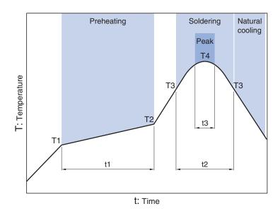
Preheating Soldering Peak Temp. Temp. Time Temp. Time Time T2 T3 T4 t3 150°C 180°C 60 to 120s 230°C 30s 260°C 10s
