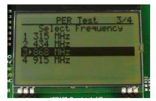
Select which frequency to use for the test. Make sure that the evaluation modules you have match the selected frequency.
