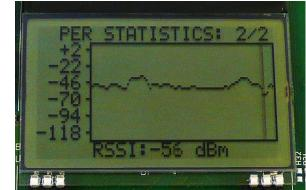
When selecting "Start PER Test", the master Press the "Up" button to go to the detailed statistical window.
