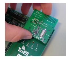
Insert a CC110LEM into the TrxEB. The connectors will only fit in one position so that the EM cannot be inserted the wrong way. Do not use excessive force on the EM.
