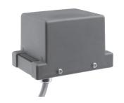
**Uncommon sense.** Honeywell Sensing and Control (S&C) offers environmentally sealed proximity sensors in a variety of technologies — including Eddy Current Killed Oscillator (ECKO) and Hall-effect. Once a metallic object is detected in front of the sensing face, a signal is passed through the conditioning circuitry to give an output configured according to the sensor application.
