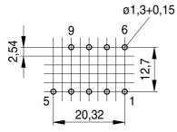
Hole arrangement View in mounting direction
