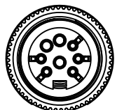
AISG 8-pin female interface with 5 loaded contacts
