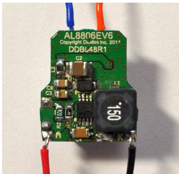
Figure 8. AL8806EV6 Evaluation Board (Top)
