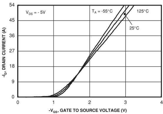
Figure 5. Transfer Characteristics.
