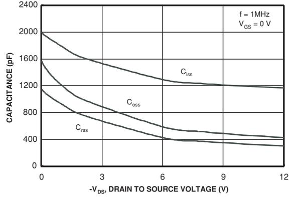
**Figure 8. Capacitance Characteristics.**
