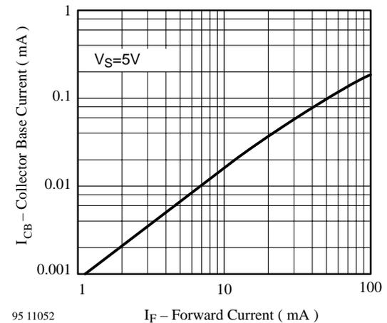
Figure 10. Collector Base Current vs. Forward Current
