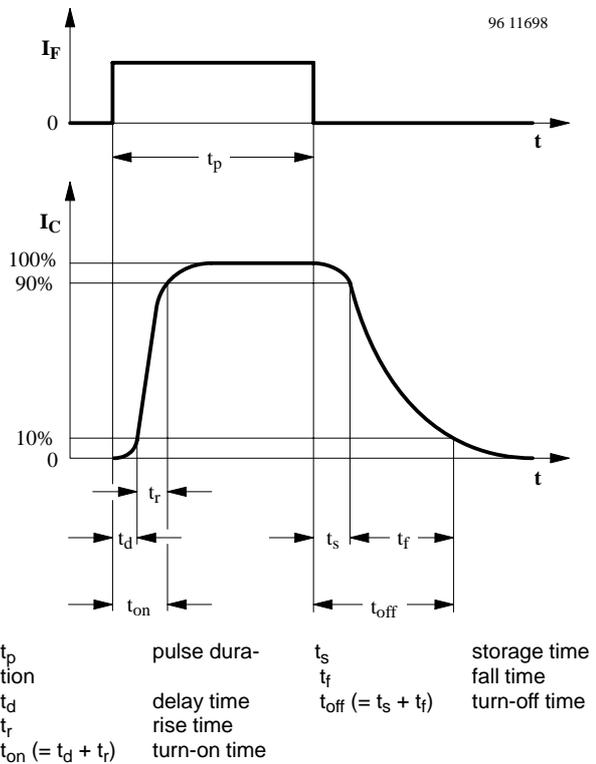
Figure 5. Switching times
