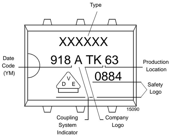
Figure 18. Marking example
