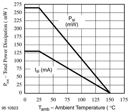
Figure 1. Derating diagram
