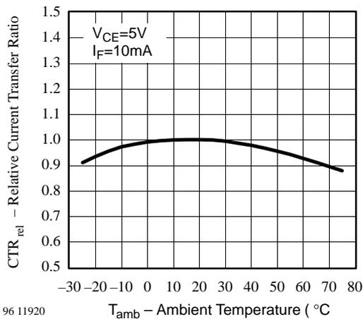
Figure 8. Relative Current Transfer Ratio vs. Ambient Temperature
