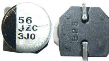
Type HZC hybrid capacitors are a combination of solid polymer aluminum technology with wet aluminum electrolytic technology. This results in a surface mount capacitor with a 4,000 hour life, low leakage current, high voltage capability, very low esr and small case sizes. They are ideal for high temperature and high reliability PC board designs. The vertical cylindrical cases facilitate automatic mounting and feature high reflow soldering temperature capability. Type HZC is RoHS compliant.
