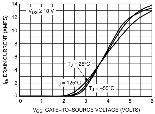
Figure 2. Transfer Characteristics
