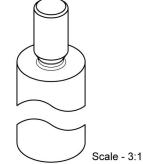
Technical Tolerances according to DIN ISO 2768m In tape & reel packaging a cap is fixed to the product to realize automatic assembly
