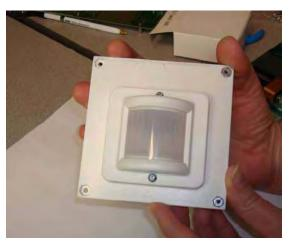
Figure 10. Assembled Flat 0.9" Lens Holder and Flat Lens
