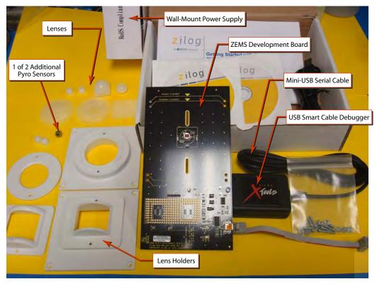
Figure 1. ZMOTION Detection and Control Development Kit Contents
