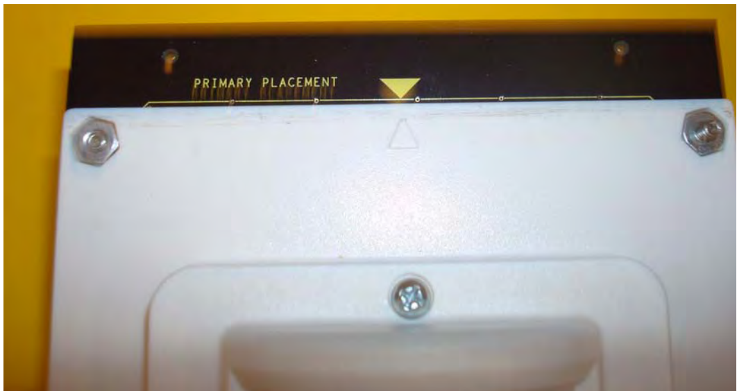
Figure 6. Top of Lens Holder on the ZMOTION Development Board
