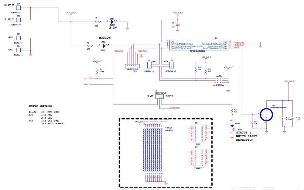
Figure 18. ZMOTION Development Board Schematic Diagram, #2 of 2
