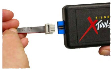
Figure 11. Connecting the Six-Conductor Ribbon Cable to the USB Smart Cable
