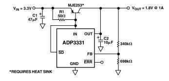
Figure 5. High Output Current Linear Regulator
