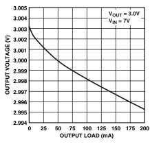
TPC 2. Output Voltage vs. Load Current
