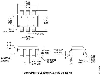
Figure 6. 6-Lead Small Outline Transistor Package [SOT-23] (RJ-6) Dimensions shown in millimeters
