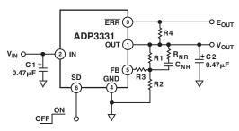
Figure 3. Noise Reduction Circuit
