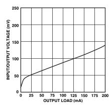
TPC 7. Dropout Voltage vs. Output Current
