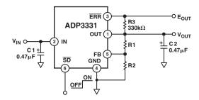
Figure 1. Typical Application Circuit
