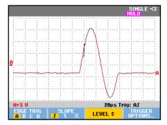
Figure 30. Making a Single Shot Measurement
