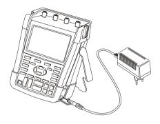
Figure 46. Charging the Batteries
