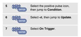
The test tool is now prepared to trigger on narrow pulses only. Observe that the trigger key labels at the bottom of the screen have been adapted to set the pulse conditions:
