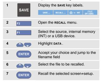
Observe that the recalled waveform is displayed and that **HOLD** appears on the screen. From this point you can use cursors and zoom for analysis or you can print the recalled screen.
