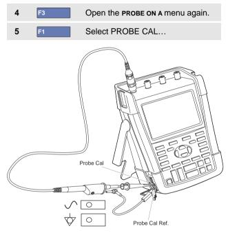
Figure 50. Adjusting Voltage Probes
