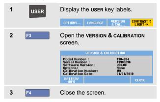
The screen gives you information about the model number with software version, the serial number, the calibration number with latest calibration date, and installed (software) options.
