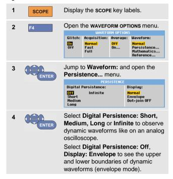
Select **Display: Dot-join: Off** to display measured samples only. Dot join off may be useful when
