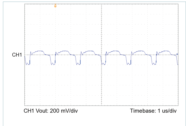
Figure 19 — Output voltage ripple, V_{IN} = 30\text{ V} , V_{OUT} = 5.0\text{ V} , C_{OUT\_EXT} = 1000\text{ }\mu\text{F} , R_{LOAD} = 0.313\text{ }\Omega
