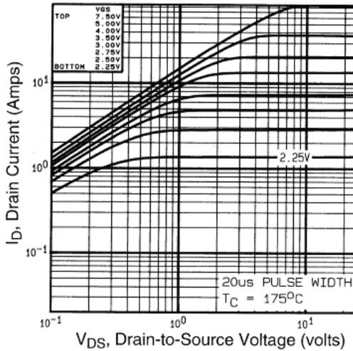
Fig. 2 - Typical Output Characteristics,  $T_C = 175\text{ }^\circ\text{C}$
