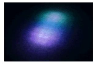
The paper acts like a rear-projection screen. In signal processing terms, it's also acting like a low-pass filter (https://adafru.it/cWb) or blur. The hard edges of each LED are filtered out, and the result looks much more like what appears on-screen.
