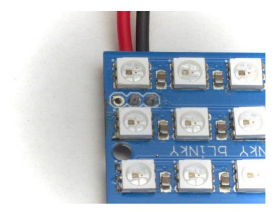
I also like to put a little solder on the other side, where the wires come out. This adds a little mechanical strength, making the wires less likely to break.
