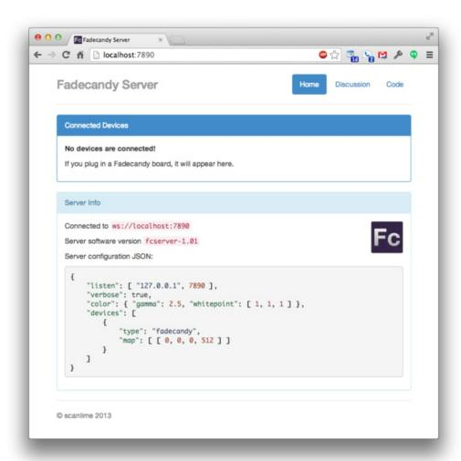
If you plug in a Fadecandy Controller board, it should show up in the *Connected Devices* section. No need to reload the web page.
