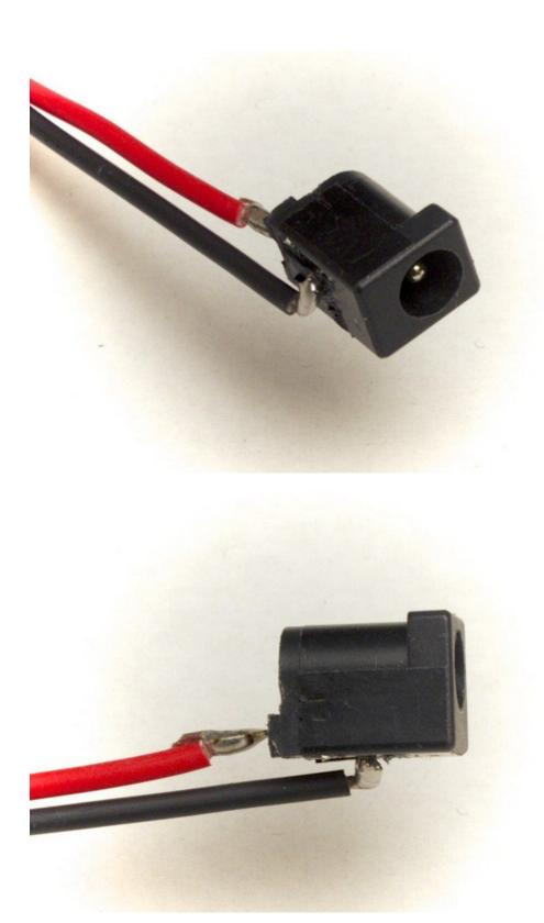
The barrel jack is almost ready to use! You'll want to insulate it, though, so you don't have to worry about metal objects bridging the two power terminals. It's especially important to watch out for short circuits when you're using such a large power supply!
