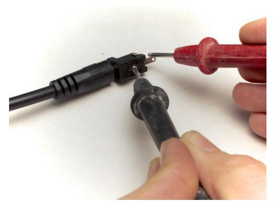
Following the polarity on the diagram above, we'll put the black probe on the pin that attaches to the outside casing of the plug, and the red probe goes on the center pin. If all is well, you should see a positive number close to 5V.
