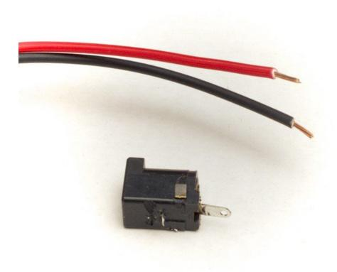
If you have multiple colors of wire, the tradition is to use black or green for ground and red or another bright color for positive. I used red and black wire. This wire should be relatively thick, since it has to carry several amps of power. I used 20 gauge stranded wire.
