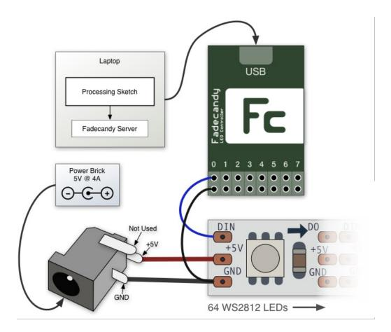
So, let's start with power. We're using a barrel jack (http://adafru.it/373) that matches the plug on our power brick (http://adafru.it/658). These jacks have three pins. The one on the side isn't used here, it's just for detecting when a plug has been inserted. The other two pins connect to the outside casing of the barrel plug, and the center pin. In the most common arrangement, this outside shell is negative (ground) and the inner pin is positive.
