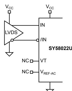
**Figure 3c. LVDS Input Interface**
