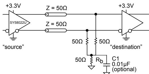
**Figure 5. Three-Resistor "Y-Termination"**
