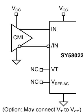
**Figure 3d. AC-Coupled CML Input Interface**
