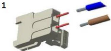
**1** - Insert stripped & tinned wires (20-22 AWG) into cavities. Be sure to push in as far as possible. Gently pull back on wires to ensure that wires are locked into place.
