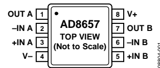
Figure 1. AD8657 Pin Configuration, 8-Lead MSOP
