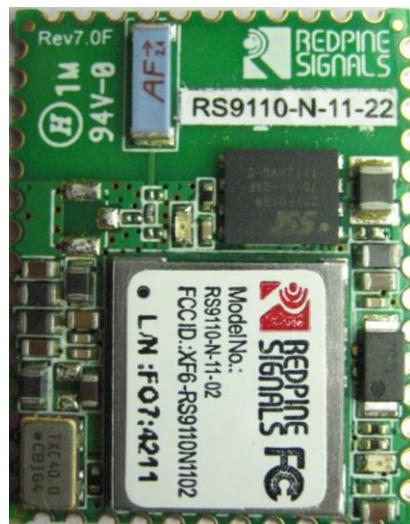
**Figure 1:Top View of the Module**
