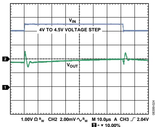
Figure 28. Line Transient Response, Load Current = 1 mA
