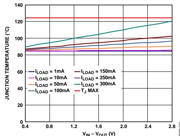
Figure 44. Junction Temperature vs. Power Dissipation,
