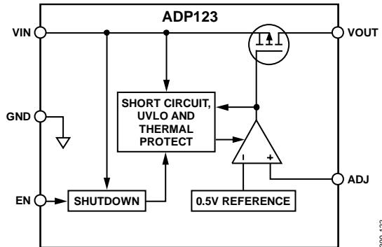
Figure 31. ADP123 Internal Block Diagram (Adjustable Output)
