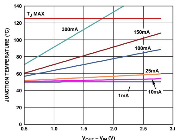
Figure 48. Junction Temperature vs. Power Dissipation,
