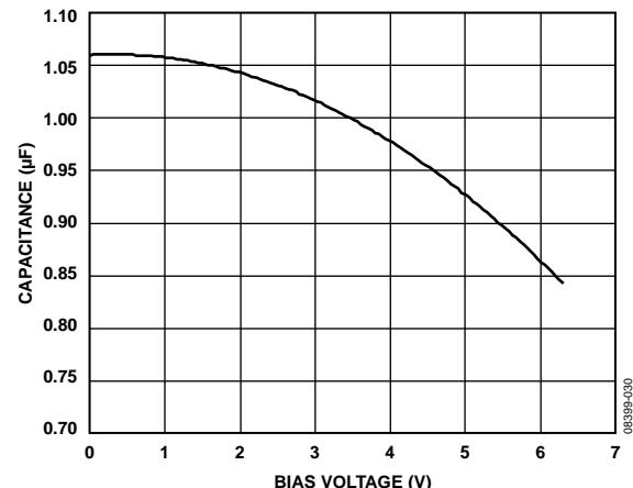
Figure 34. Capacitance vs. Capacitor Voltage Bias Characteristics
