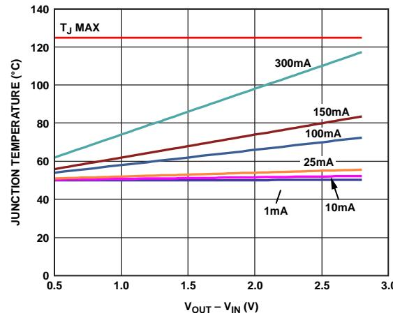
Figure 47. Junction Temperature vs. Power Dissipation,
