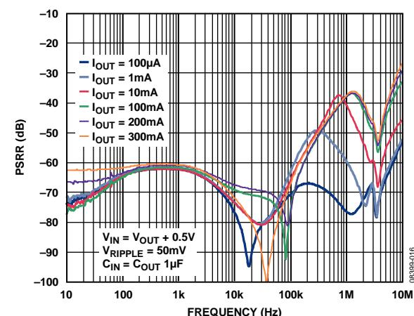
Figure 20. Power Supply Rejection Ratio vs. Frequency,  $V_{\text{OUT}} = 3.3\text{ V}$ ,  $V_{\text{IN}} = 3.8\text{ V}$
