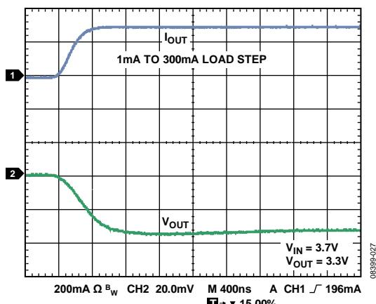
Figure 33. Output Transient Response,  $C_{\text{OUT}} = 4.7 \mu\text{F}$
