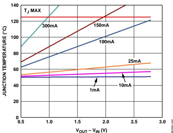
Figure 50. Junction Temperature vs. Power Dissipation,
