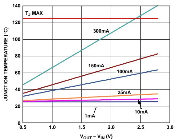
Figure 46. Junction Temperature vs. Power Dissipation,
