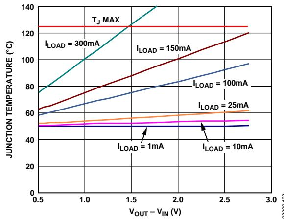
Figure 43. Junction Temperature vs. Power Dissipation,
