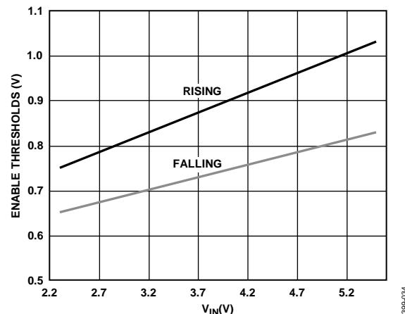
Figure 36. Typical EN Pin Thresholds vs. Input Voltage
