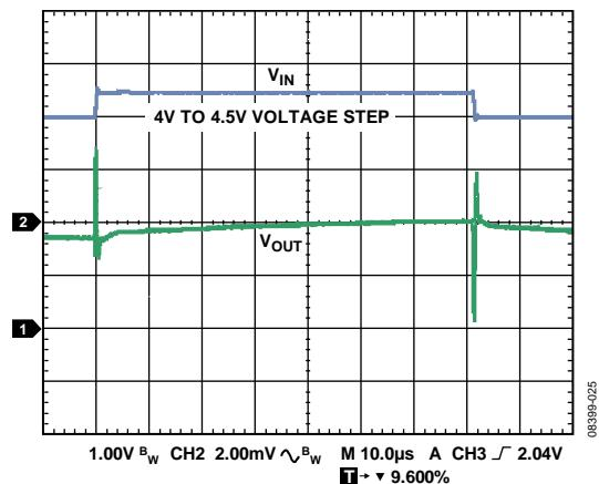
Figure 29. Line Transient Response, Load Current = 300 mA
