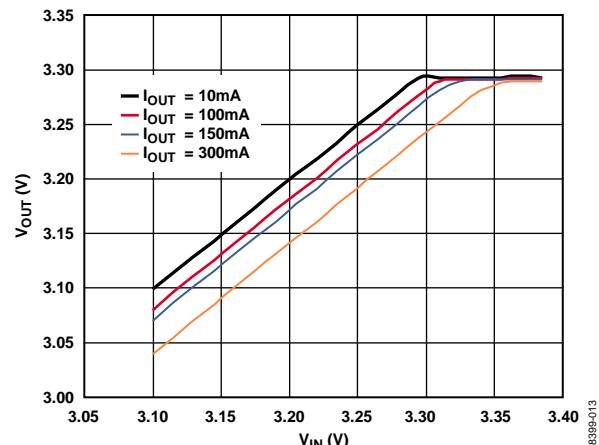
Figure 18. Output Voltage vs. Input Voltage (in Dropout)
