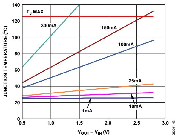
Figure 49. Junction Temperature vs. Power Dissipation,
