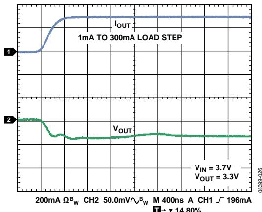
Figure 32. Output Transient Response,  $C_{\text{OUT}} = 1 \mu\text{F}$
