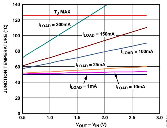
Figure 42. Junction Temperature vs. Power Dissipation,
