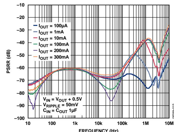
Figure 19. Power Supply Rejection Ratio vs. Frequency,  $V_{\text{OUT}} = 2.8\text{ V}$ ,  $V_{\text{IN}} = 3.3\text{ V}$
