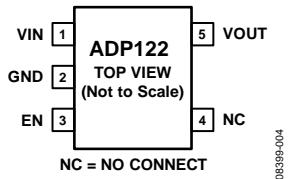
Figure 5. ADP122 TSOT Fixed Output Pin Configuration
