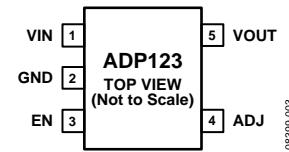
Figure 7. ADP123 TSOT Adjustable Output Pin Configuration
