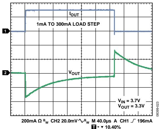
Figure 27. Load Transient Response,  $C_{OUT} = 4.7 \mu F$
