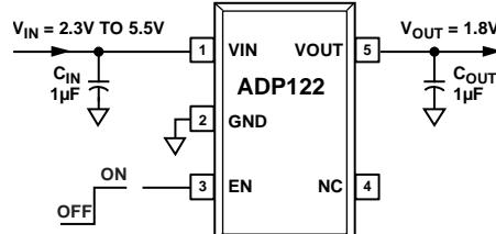
Figure 1. ADP122 with Fixed Output Voltage (TSOT Version)
