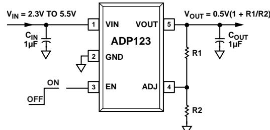
Figure 2. ADP123 with Adjustable Output Voltage (TSOT Version)
