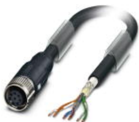
Bus system cable, VARAN, 6-position, PVC, black, shielded, free cable end, on Socket straight M12 SPEEDCON, A-coded, cable length: 1.5 m, Customer version
