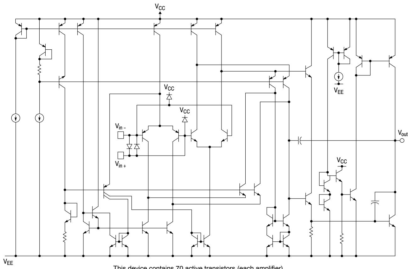
**Figure 1. Circuit Schematic
