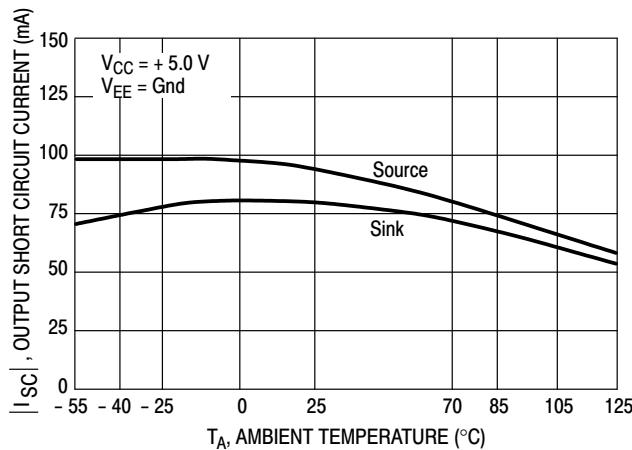
**Figure 14. Output Short Circuit Current versus Temperature**
