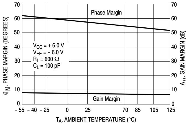
**Figure 20. Gain and Phase Margin versus Temperature**
