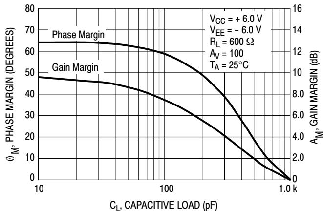
**Figure 22. Gain and Phase Margin versus Capacitive Load**
