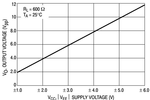
**Figure 8. Output Voltage Swing versus Supply Voltage**
