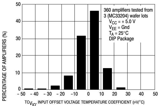
**Figure 4. Input Offset Voltage Temperature Coefficient Distribution**
