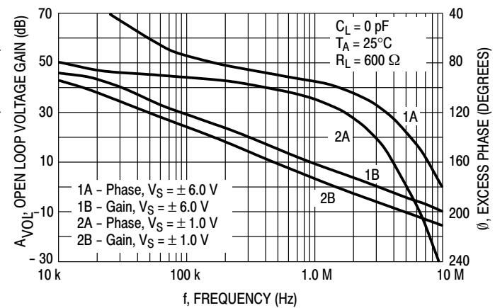
**Figure 19. Voltage Gain and Phase versus Frequency**
