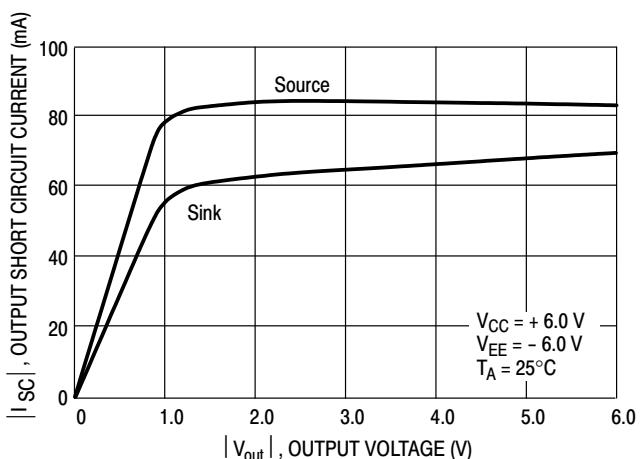
**Figure 13. Output Short Circuit Current versus Output Voltage**
