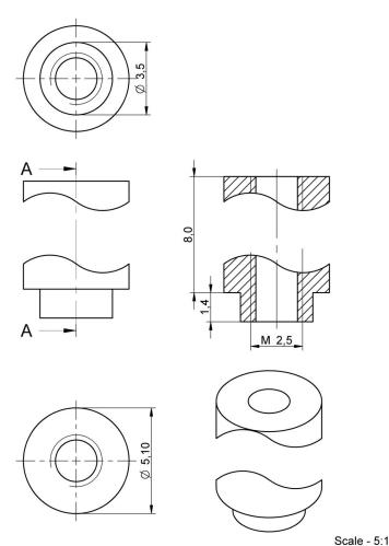
Technical Tolerances according to DIN ISO 2768m
