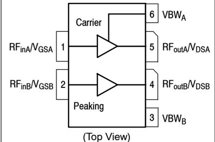
Figure 1. Pin Connections
