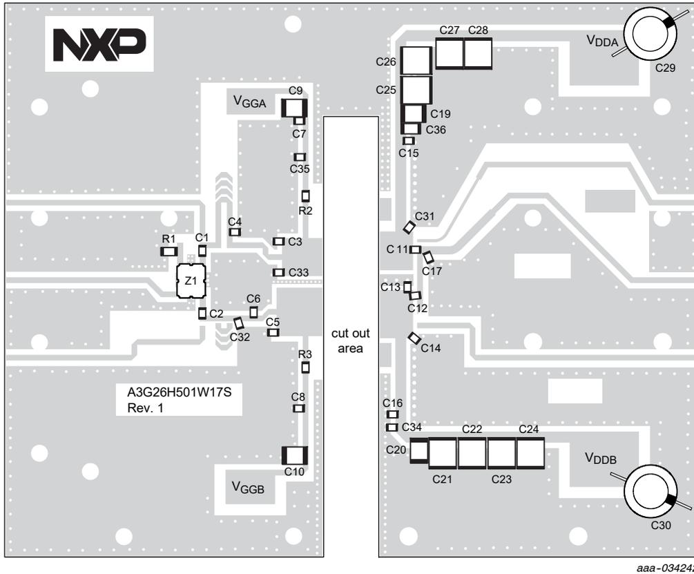
Figure 2. A3G26H501W17S Production Test Circuit Component Layout
